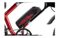
2. **Test the battery lock security.** Ensure key port is aligned with the circle containing an "X," in the "Locked" position indicating locked onto the frame mount. If needed, insert the key and align with the "Locked" icon. Remove the key and carefully use both hands to pull up on the battery to test that the lock is secure.
