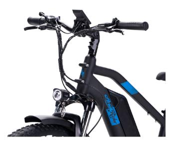
Before securing the handlebars completely, rotate the bars so that the brake levers angle downward at an angle of 40-45°. The stem angle (handlebar height) is adjustable. If the angle is adjusted, be advised to always keep the stem angle leaning forward for stability purposes. (Don't adjust it to straight up and down!)
