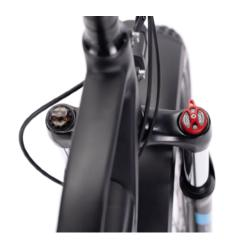
In most situations, it is best to leave the suspension unlocked. When locked, the suspension can no longer absorb the various impacts and vibrations encountered while riding, and as a result those forces are transferred directly to the rider. This also puts more strain on parts such as the wheels, and handlebar stem.
