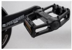
The right pedal is threaded so that it is tightened by turning clockwise, has an "R" stamped into the pedal axle end, and a smooth exterior on the outside of the pedal axle. Carefully thread the right pedal onto the crank on the right side of the bike (the side with the drive train) slowly and by hand.
