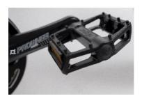
The right pedal is threaded so that it is tightened by turning clockwise, has an "R" stamped into the pedal axle end, and a smooth exterior on the outside of the pedal axle (2, above). Carefully thread the right pedal onto the crank on the right side of the bike (the side with the drivetrain gears) slowly and by hand. Do not cross thread or damage the threads. Tighten securely using a pedal wrench to avoid damage caused by wider wrenches.
