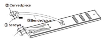
(6)The integration of solar energy lamps set into the lamp, use a special tool for fastening screws, ensure
