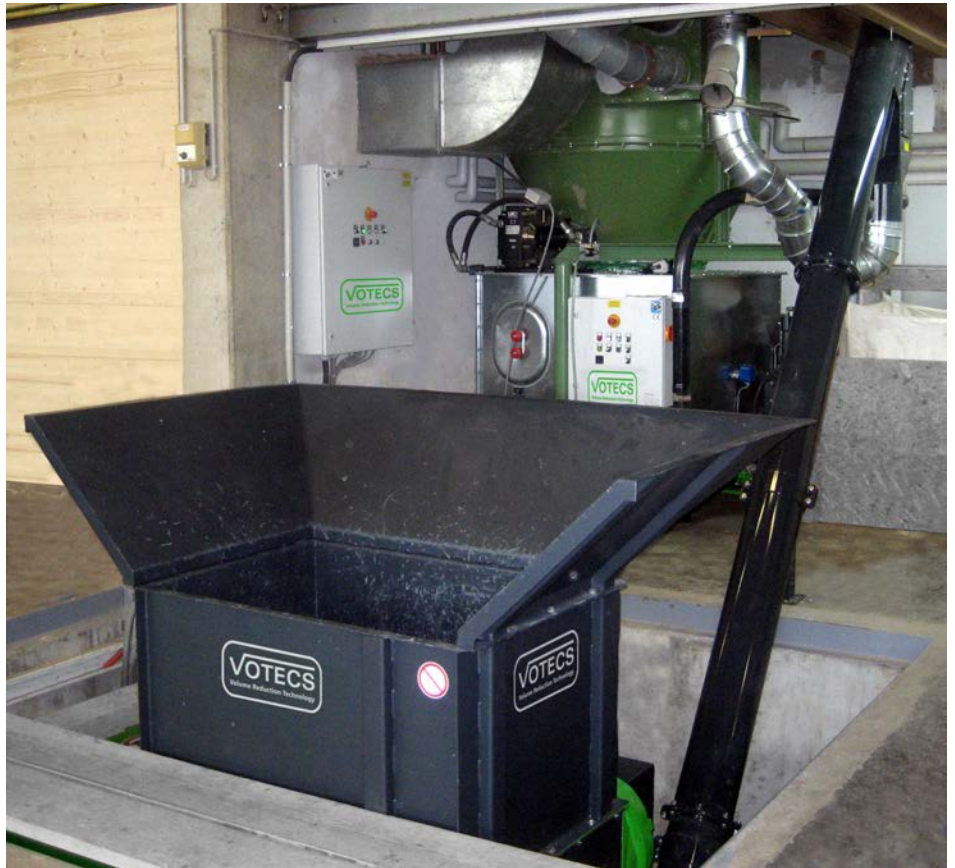
Shredder EZ 8/2 installed in a pit. Material transport by a 11 meters ascending worm screw going up to silo filling.
