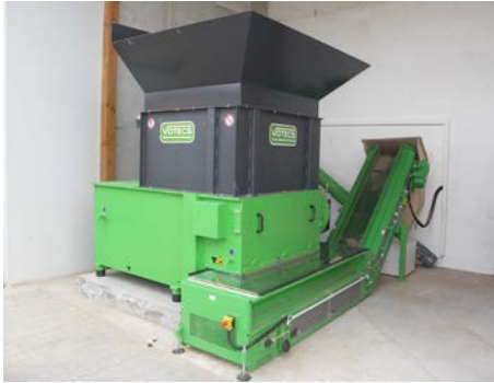
Shredder EZ 8/2 installed in a pit. Material transport by a 11 meters ascending worm screw going up to silo filling.
