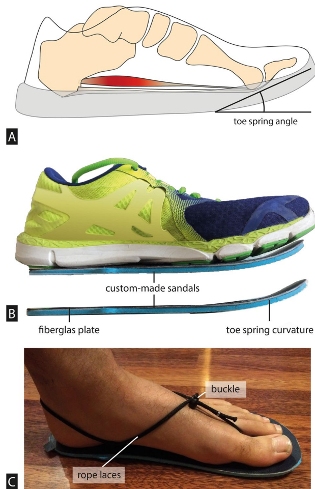
Figure 1. A toe spring describes the curve upward of the sole of a shoe. (A) The upward curvature below the metatarsal heads orients the toe box dorsally relative to the rest of the shoe. (B) Custom-made sandals with varying degrees of toe spring angle were manufactured to mimic the stiffness and shape of toe springs commonly found in commercially available shoes. (C) The sandals were secured with minimal rope laces that could be adjusted by a buckle and did not restrict the placement of reflective markers.
