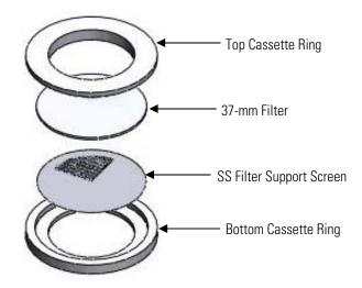
Figure 5–2. Filter Cassette Assembly – Snap Rings and Filter
