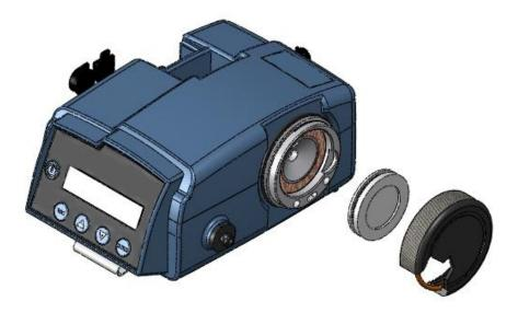
**Figure 5–1.** Filter Assembly Location – turn counter-clockwise to open Replacement of the o-ring is to also be maintained in order to provide an adequate seal (see Figure 5–2).
