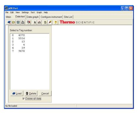
In this second image of the Data Text tab, it shows a Tag File loaded to the window. The data can now be viewed in the Data Graph tab and saved as a CSV file.
