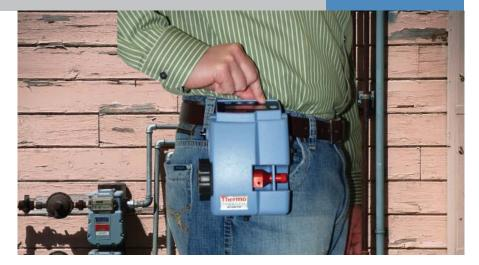
The Thermo Scientific pDR-1500 personal DataRAM was developed to meet the need for a fully integrated, active sampling personal scale instrument with greater accuracy, increased capabilities, low size and weight, maximum ease-of-use and increased operating time.
