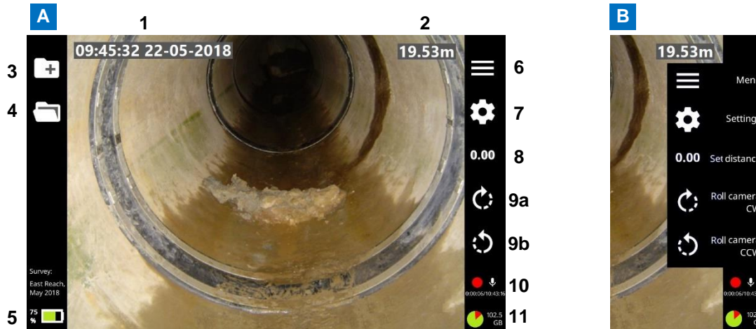
Fig. 3.7: Controller home screen. A Button labels hidden. B Button labels shown. See next page for descriptions.
