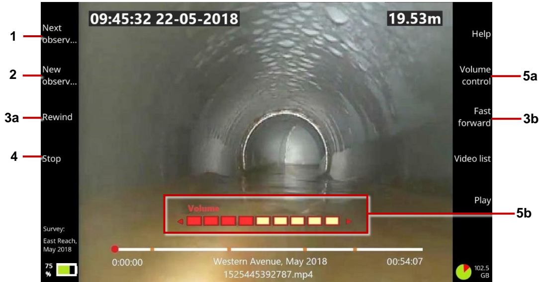
Fig. 6.7: Video playback screen. 1 Next observation button. 2 New observation button. 3a, 3b Rewind and Fast Forward buttons. 4 Stop button. 5a Volume Control button. 5b Volume level Use the ⇐ ⇨ arrow keys to adjust the volume.
