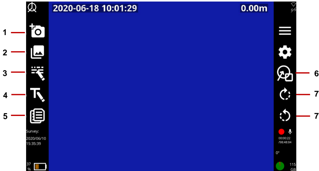
Fig. 7.2: Edit survey screen. 1 New observation button. 2 List observations button. 3 Edit survey header button. 4 Title page button. 5 Text pages button. 6 Overlay graphics button (for observations). 7 Roll camera buttons.
