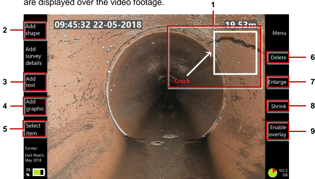
Fig. 6.6: Adding overlay items to a video recording. 1 Overlay text and shapes. Buttons: 2 Add shape. 3 Add text. 4 Add graphic. 5 Select item. 6 Delete item. 7 Enlarge item. 8 Shrink. 9 Enable overlay / Disable overlay.
