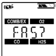
Figure 3-1. Fresh Air Setup
