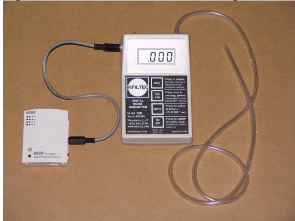
Figure 1 – DM1 micro-manomter, Analog Data Cable, Onset U12-012, ¼” Pressure connect tubing
