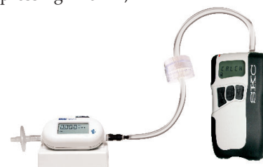
Calibration train with sample medium in line
