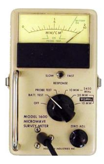
Turn the selection knob on the meter to the "PROBE TEST" position. With the "ZERO ADJ." knob in a center position, the meter should read between the green lines (in the "OK PROBE TEST" area). If it does not, the probe has been damaged and should not be used. A defective probe cannot be replaced in the field and should be returned to ETS-Lindgren for repair. See the Product Information Bulletin included with your shipment for details regarding returning instruments for repair.
