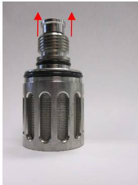
Figure 4-7b: Removing Check Ball Retainer
