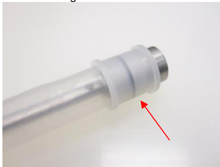
Figure 4-15: Bottom Compression ring with visible O-ring
