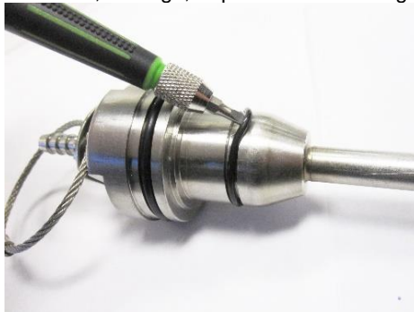
Figure 4-5: Removal of O-rings
