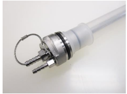
Figure 4-14b: Compression ring secured
