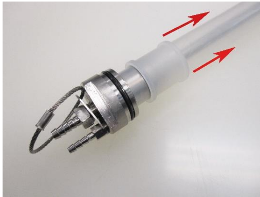
Figure 4-3: Removal of upper Compression Ring
