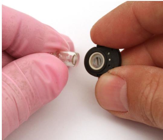
Figure 31: Reinstalling the Electrode Lamp
