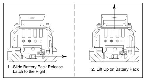
Figure 13: Releasing the Battery Pack
