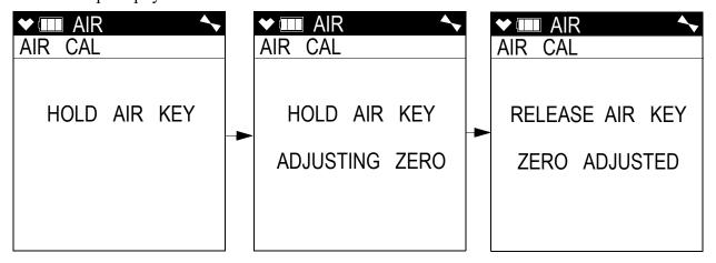
9. Release the ▲ AIR button. The fresh air adjustment will finish, the fresh air reading will be displayed momentarily, and then the instrument will return to the Calibration Mode Screen.
