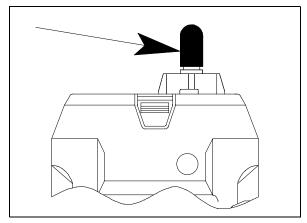
6. Reconnect the tubing to the open end of the dehumidifier filter to help preserve its life. If the filter begins to appear wet, it needs to be replaced.
