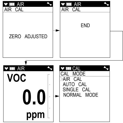
7. If the VOC zero filter was used, remove the filter from the GX-6000's inlet fitting or probe. Reinstall the plugs on each end of the filter.
