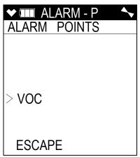
3. Press and release POWER/ENTER. The channel's alarm points are displayed.
