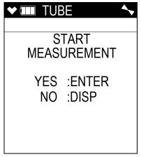
7. Press and release the POWER/ENTER button to start the benzene measurement.
