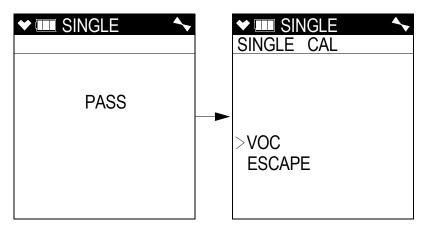
14. Press and release the POWER/ENTER button to save the span value. The LCD will indicate that the calibration has ended, then the Select Sensor Screen appears.
