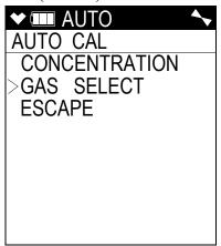
14. Press and release the POWER/ENTER button. The PID sensor screen will be displayed. In addition to the PID sensor screen, there is an **ESCAPE** screen that will take you back to the Auto Cal menu. Use the ▲ AIR and SHIFT ▼ (PANIC) buttons to scroll between the screens.
