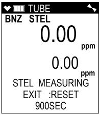
d. To cancel the STEL measurement, press and release the RESET button. Then press and release the POWER/ENTER button.
