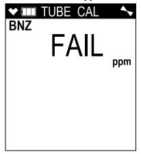
Press and release the RESET button to clear the alarm and return to the TUBE CAL Auto Calibration Menu. See "Troubleshooting" on page 93.
