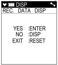
3. Press and release the POWER/ENTER button. The screen that appears will depend on whether or not any data has been saved to the snap logger.
