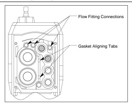
Figure 35: Sensor Gasket Seating
