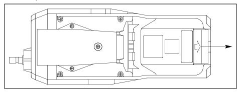
Figure 10: Releasing Battery Cover Latch
