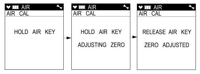
6. Release the ▲ AIR button. The fresh air adjustment will finish, the fresh air reading will be displayed momentarily, and then the instrument will return to the Calibration Mode Screen.
