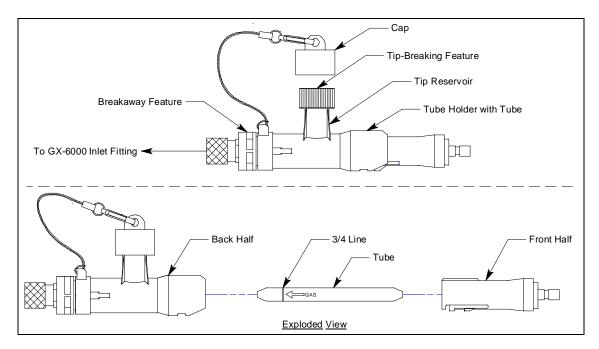
**Figure 36: Tube Holder Component Location**
