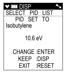
1. With the PID Gas Name Screen displayed, press and release the POWER/ENTER button. The top level of the PID Gas Name List will be displayed and the cursor will be next to the letter corresponding to the first letter of the current setting. In the example below, the PID channel is configured for isobutylene so the cursor is next to "I". Each letter has a list of gas names behind it.
