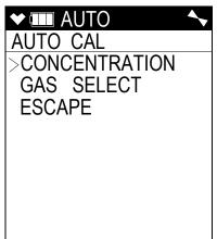
6. To check or update the gas concentration, use the ▲ AIR and SHIFT ▼ (PANIC) buttons to put the cursor next to **CONCENTRATION** and press and release the POWER/ENTER button to display the Calibration Gas Values Screen.
