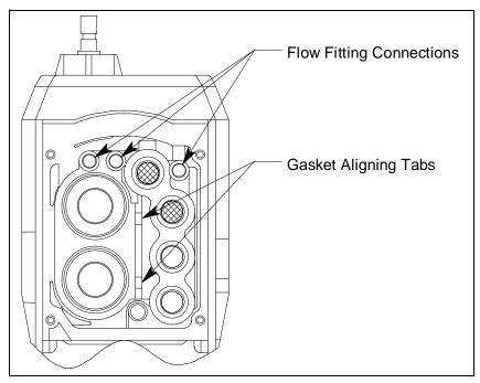
Figure 23: Sensor Gasket Seating
