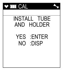
4. Be sure a filter tube is installed in the tube holder and then attach the tube holder to the instrument's inlet fitting. See page 181 for instructions.
