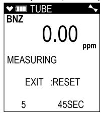
9. To cancel the measurement, press and release the RESET button.
