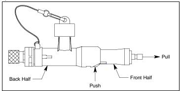
Figure 37: Replacing a Tube
