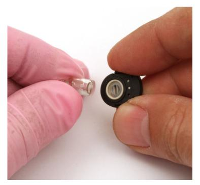
Figure 34: Reinstalling Electrode Lamp
