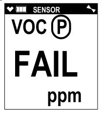
The GX-6000 cannot be used if the PID sensor fails. Turn the instrument off and replace the sensor.
