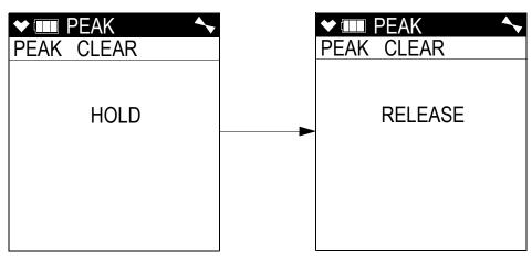
2. Release the RESET button. The peak reading will be reset and the unit will return to the Peak Screen.
