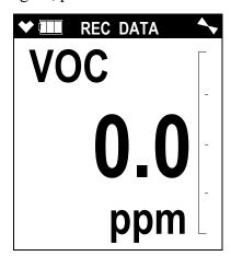
The gas reading that was taken during the snap log is displayed. You can use the ▲ AIR and SHIFT ▼ (PANIC) buttons to scroll through the different snap logs. The gas reading will change as you view different snap log data but the snap log ID is not visible from this screen. To scroll through the data by viewing the snap log ID number, press and release POWER/ENTER.
