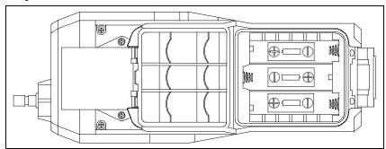
Figure 12: Installing the Alkaline Batteries
