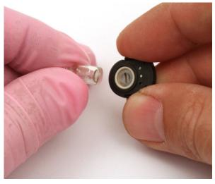
Figure 28: Reinstalling the Electrode Lamp
