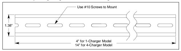
**Figure 4: DIN Rail Dimensions**
