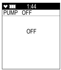
2. To turn the pump back on and continue in Display Mode or return to Measuring Mode, press and release the DISP/LOCK button.
