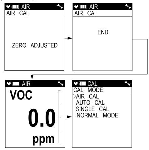
10. If the VOC zero filter was used, remove the filter from the GX-6000's inlet fitting or probe. Reinstall the plugs on each end of the filter.
