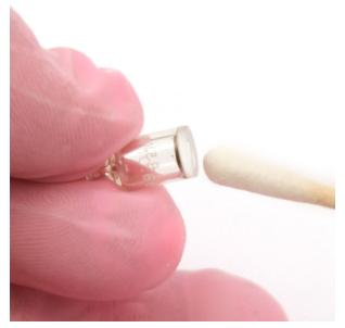
Figure 27: Polishing the Electrode Lamp Window
