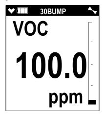
If you do not want to proceed with the bump test, press and release the DISP/LOCK button to return to the Gas Select Screen.
