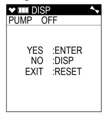
1. In this screen, press and release the POWER/ENTER button to turn the pump off. The fan symbol in the upper right corner will disappear. Once the pump is off, you cannot exit this screen and return to Measuring Mode or continue in Display Mode until you turn the pump back on.
