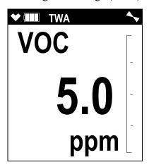
The TWA reading is the average reading *over the last 8 hours*. If 8 hours have not elapsed since the last time the TWA reading was cleared, the average is still calculated over 8 hours. The missing time is assigned a 0 value for readings. If **LUNCH BREAK** is set to **OFF**, the TWA is cleared when the GX-6000 is turned off.
