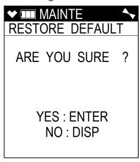
5. Press and release the POWER/ENTER button. The screen will indicate that the default configuration has been restored and return to the main menu.
