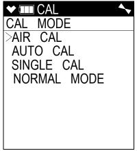
5. Press and release the POWER/ENTER button. The Fresh Air Reading screen will display.
