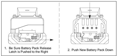
Figure 14: Installing the Battery Pack
