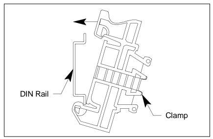
Figure 6: Clamp Installation
