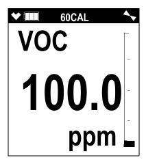
b. At the end of the calibration, the instrument displays the results from both the bump test and the calibration. Use the ▲ AIR and SHIFT ▼ (PANIC) button to scroll between the calibration/bump test results, the bump test gas reading, and the calibration gas reading.
