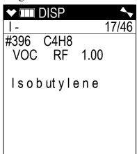
5. To select a gas name, press and release the POWER/ENTER button while you are viewing the parameters. The selection will be in effect until you change it again.
