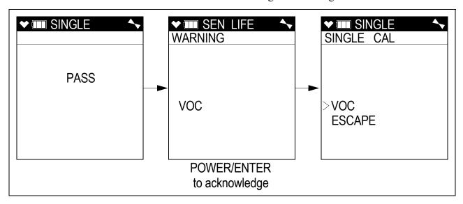
13. If the PID sensor is not in a sensor life warning condition or if **SEN LIFE ALERT** is set to **OFF** (factory setting), the following screen sequence occurs.
