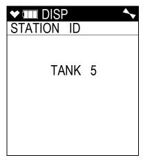
The station ID provides a way to identify a location where monitoring was done during a data logging session. See the GX-6000 Data Logger Management Program Operator's Manual for a detailed description of data logging and the station ID.
