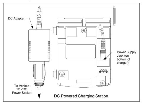
Figure 16: Connecting the Charging Station's DC Adapter
