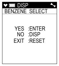
• The PID Gas Name Screen operates as described on page 45 but is factory set up for and calibrated to benzene and appears as shown below.
