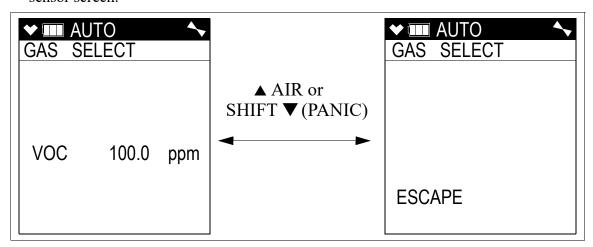
9. Before proceeding, confirm that the bump test gas value is the same as the concentration in the calibration cylinder. If it is not, adjust the bump test gas value by entering the **AUTO CAL** menu item in Calibration Mode, changing the value there, and reentering the **BUMP TEST** menu item.
