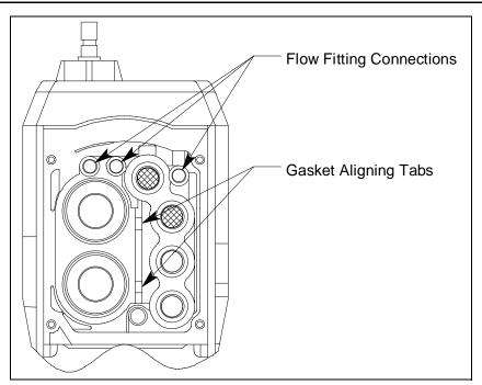
Figure 29: Sensor Gasket Seating
