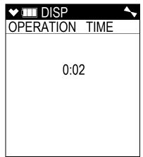
If **LUNCH BREAK** is set to **ON**, the time in operation will only be reset if you do not choose to resume the peak and TWA measurements when the GX-6000 is turned on in the Lunch Break Screen described in Step 3 on page 25. If you choose to resume the peak and TWA measurements during startup, the GX-6000 will include the time in operation when the unit was last turned off in the current time in operation.
