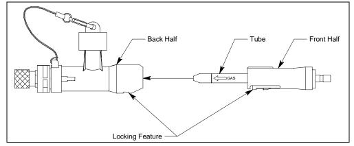
Figure 39: Reassembling Tube Holder
