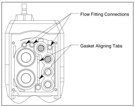
Figure 32: Sensor Gasket Seating
