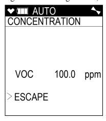
12. Press and release the POWER/ENTER button. The instrument returns to the Auto Cal Menu.
