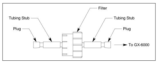
Figure 3: VOC Zero Filter
