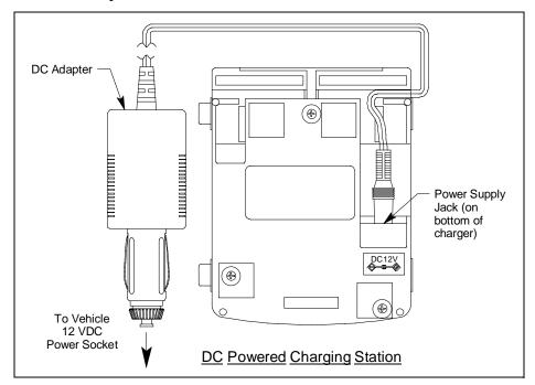
Figure 19: Connecting the Charging Station's DC Adapter
