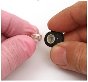
Figure 31: Reinstalling the Electrode Lamp
