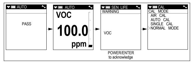
21. If the PID channel passed calibration <u>and</u> if the PID sensor is not in a sensor life warning condition or if **SEN LIFE ALERT** is set to **OFF** (factory setting), the following screen sequence occurs.
