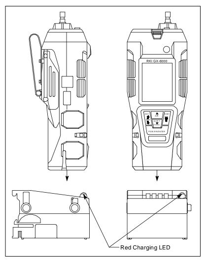
Figure 17: Putting the GX-6000 into the Charging Station
