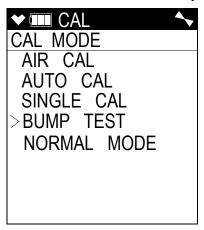
8. Press and release the POWER/ENTER button. The PID sensor screen will be displayed. In addition to the PID sensor screen there is an **ESCAPE** screen that will take you back to the Calibration Mode menu. Use the ▲ AIR and SHIFT ▼ (PANIC) buttons to display the PID sensor screen.
