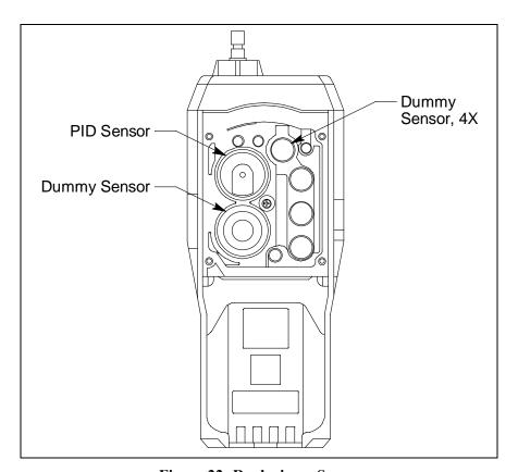
Figure 22: Replacing a Sensor
