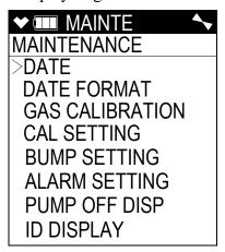
13. Use the ▲ AIR or SHIFT ▼ (PANIC) button to move the cursor up and down through the menu items. Additional items are available above and below the items currently displayed on the screen. They will appear as you scroll farther up or down the current list using the ▲ AIR or SHIFT ▼ (PANIC) buttons.
