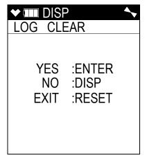
To continue through Display Mode without clearing the log data, press and release the DISP/LOCK button.
