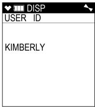
2. Use the ▲ AIR and SHIFT ▼ (PANIC) buttons to scroll through the available user IDs. The list will wrap around if you get to the top or bottom. Any of the user IDs in the list that have not been changed from the factory setting will be shown as USER\_ID\_XXX where the "XXX" is a number from 001 to 128.
