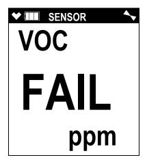
The buzzer and alarm LEDs activate in a double pulsing pattern. Press and release the RESET button to reset the alarm and continue to the Gas Select Screen. Attempt to calibrate the PID channel again. If the failure continues, investigate the cause. See "Troubleshooting" on page 93.
