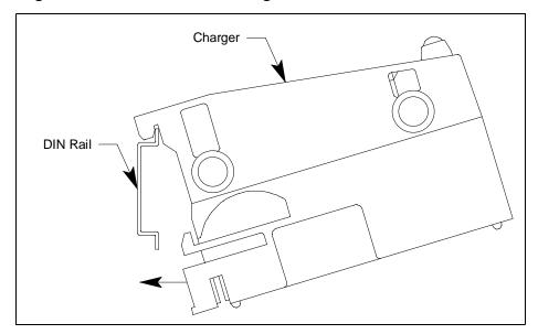
Figure 5: Installing a Charger on the DIN Rail
