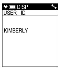
The user ID provides a way to identify the GX-6000 user during a data logging session. See the GX-6000 Data Logger Management Program Operator's Manual for a detailed description of data logging and the user ID.
