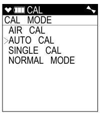
5. Press and release the POWER/ENTER button to display the Auto Cal Menu.
