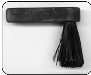
Level 2- Moderate splaying, have spare ready
