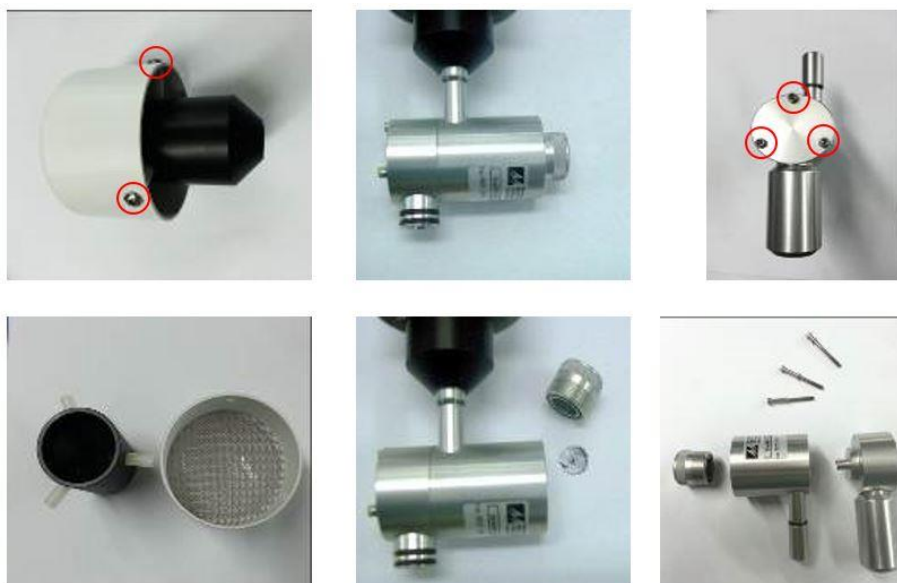
Figure 6-20 The TSP head and cyclone can be disassembled for cleaning.
