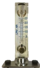
Figure 6-3 DS R8, 0.2 - 2.5 L/min rotameter for PM flow measurements.
