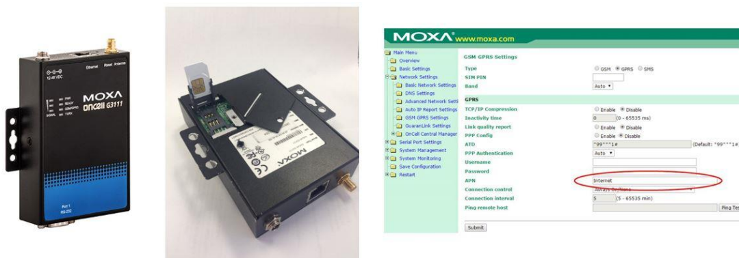
Figure 4-6 The MOXA modem uses a SIM card and it must be configured for use.
