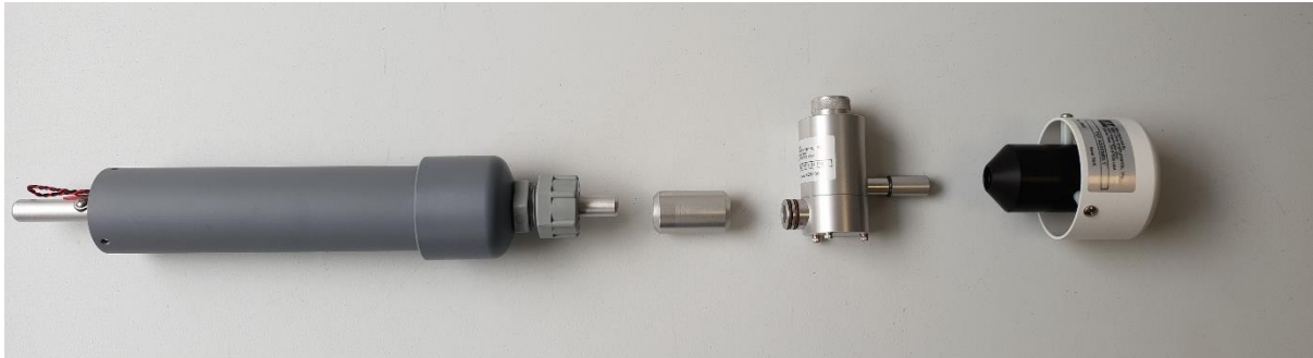
Figure 2-1 Particle sampling inlet parts including (L-R): inlet tube, cyclone adaptor, cyclone, TSP head.
