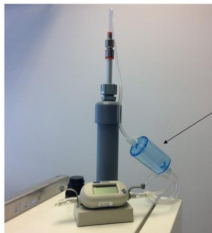
Figure 6-12 When measuring the flow on the Particle Profiler it is important to use the flow buffer chamber
