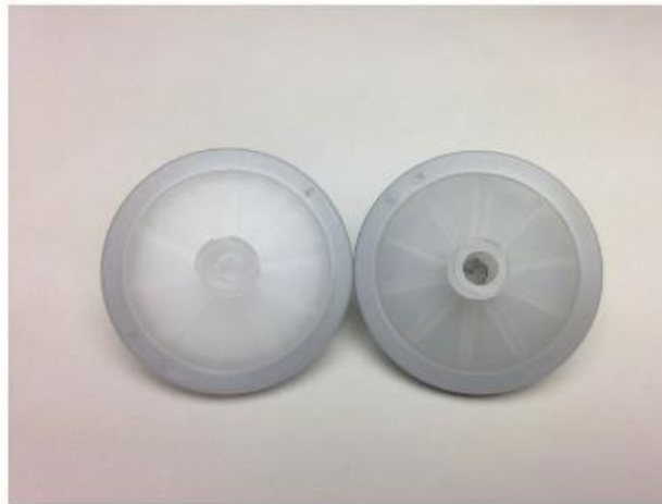
Figure 6-6 The particle filter on the gas inlet can be easily replaced, it should be replaced when it gets dirty as shown in the image on the right (a new filter is shown on the left, dirty filter on the right).
