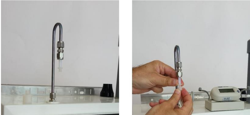
Figure 6-7 To measure the flow rate, remove the Kynar inlet filter and attach the inlet flow adaptor.
