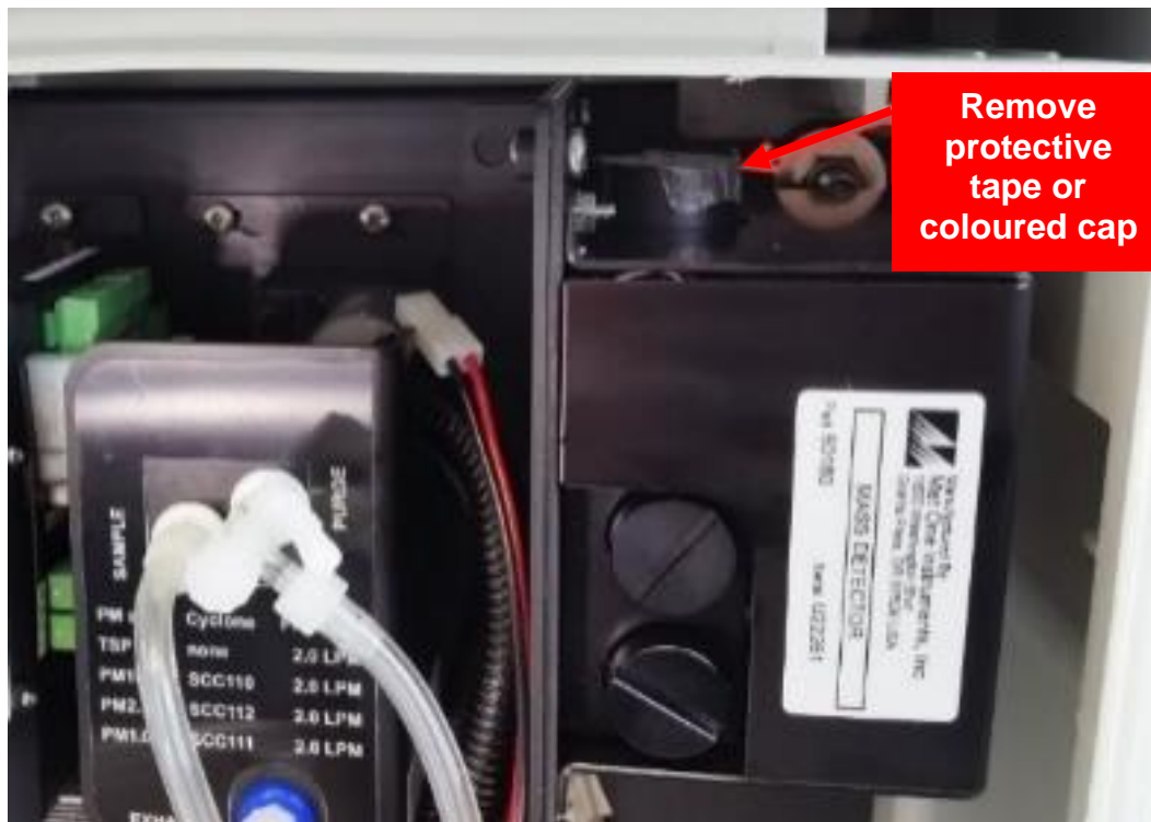
Figure 2-3 Remove the protective tape or cap from the PM inlet
