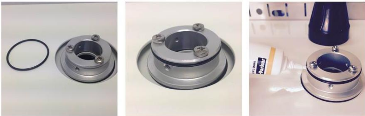
Figure 2-2 Add the O-ring and a small amount of lubricant.
