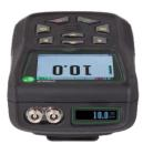
The **Cygnus 6<sup>+</sup> PRO** thickness gauge has a full range of features, including multi-mode measuring capabilities, A-scan, B-scan and comprehensive data logging.
