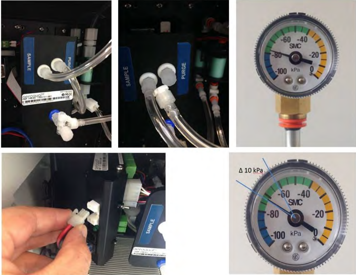
Figure 4-15 Cap the purge and exhaust lines. Place the vacuum gauge on the inlet. Disconnect the power, observe the change in pressure.
