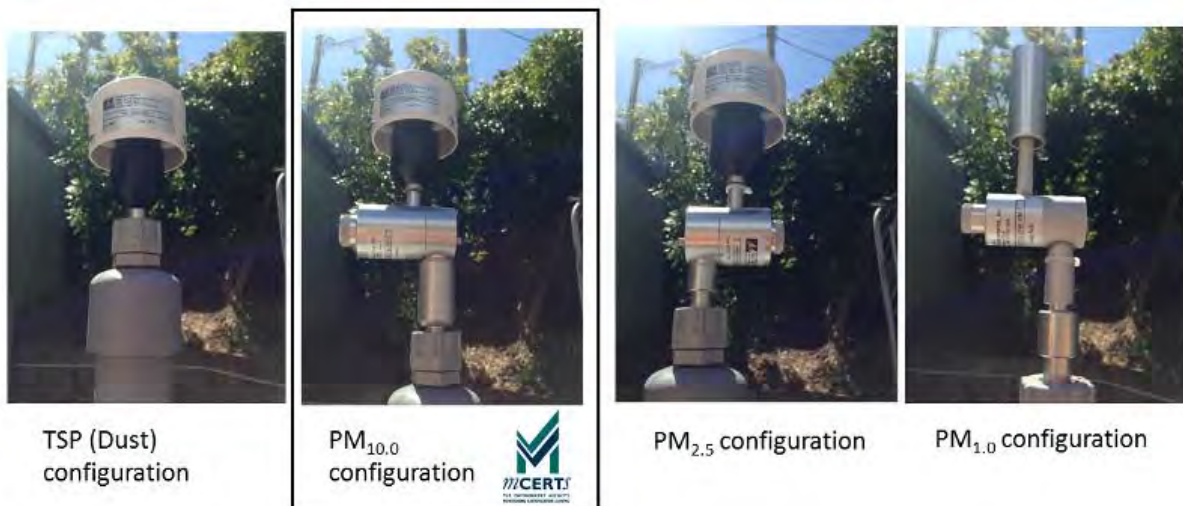
Figure 1-12 Size selection in the Particle Monitor is determined by the sharp cut cyclone on the inlet See section 4.4.7.4 for how to change the size designation in the software.
