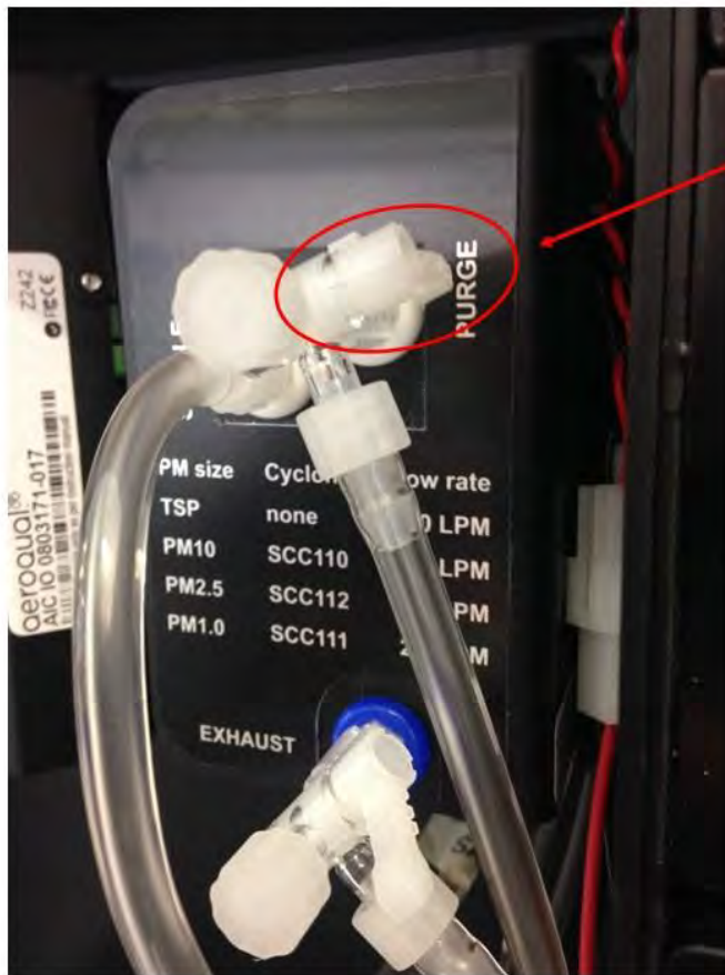
Figure 4-12 The flow rate of the Particle Monitor is set by adjusting the purge and exhaust valves
