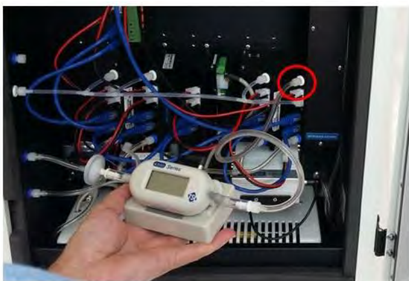
Figure 4-6 To measure the individual module flow rates, disconnect the gas inlet and attach the module inlet to the vacuum port of the R7 flow meter.
