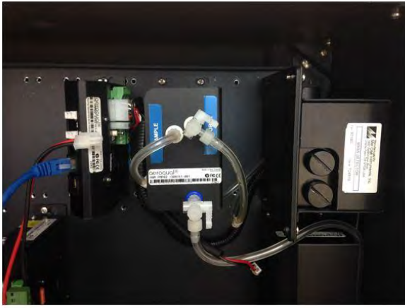
Figure 2-4 With mains power on, and with the 12 V DC fuse pulled out, there should be air flow coming from the top of the AQM as shown on the right. Disconnect the power (red/back) cable from the PM pump module while testing the power, as shown on the left
