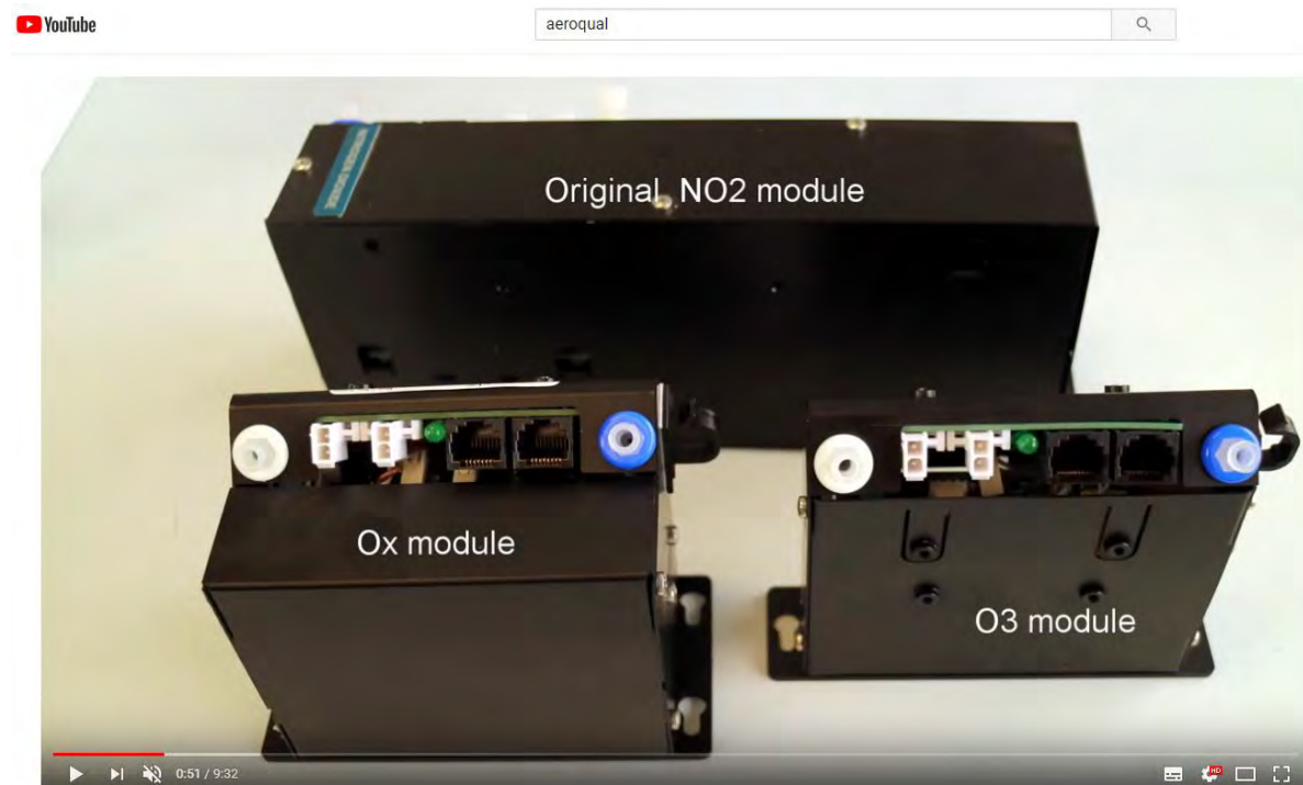
Figure 1-5 Replacing NO 2 module with O x /O 3 system for measuring NO 2
