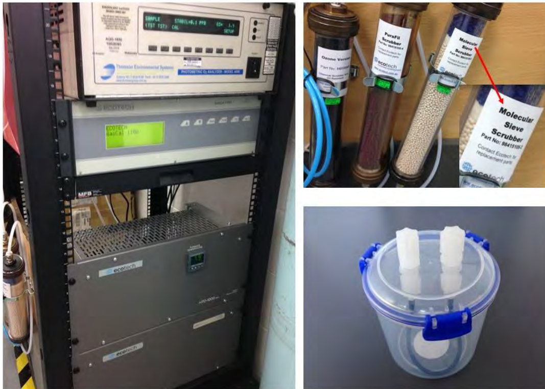
Figure 7-3 Left: Ecotech and Teledyne calibration system. Top Right: Drying agent molecular Sieves. Bottom right: Aeroqual R41 humidifier.
