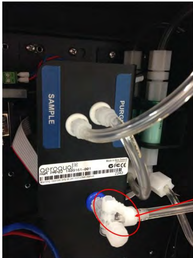
Figure 4-13 The flow rate of the Particle Profiler is set by adjusting the flow adjustment valve
