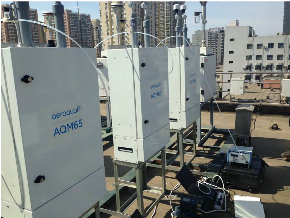
Figure 5-4 The Ozone calibrator and AirCal 1000 can calibrate multiple instruments at the same time.
