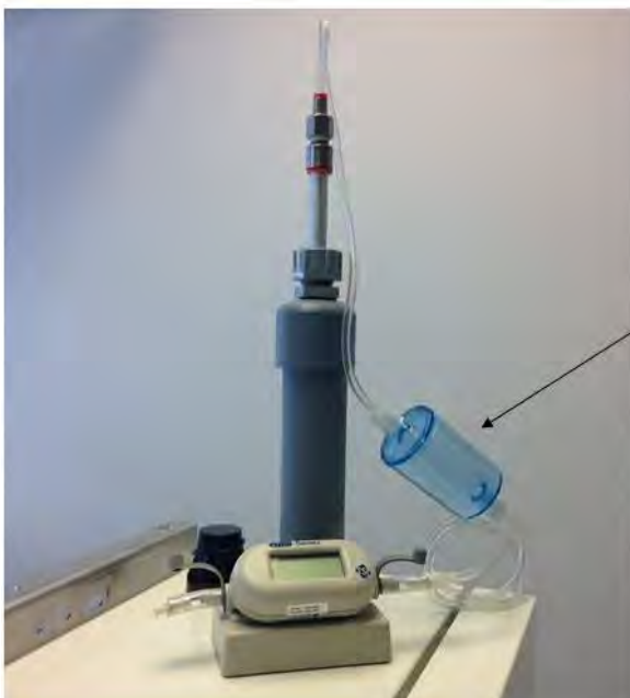
Figure 4-11 When measuring the flow on the Particle Profiler it is important to use the flow buffer chamber
