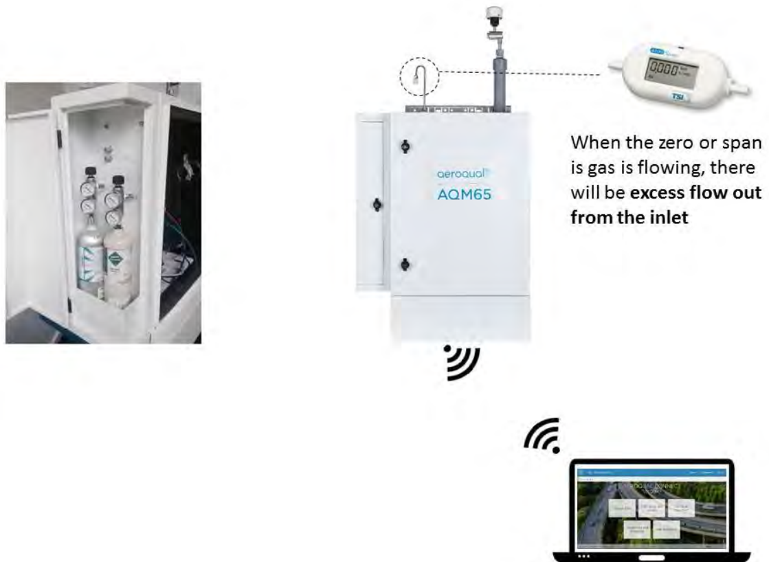
Figure 5-14 Setup to perform a zero and span calibration using the AirCal 8000
