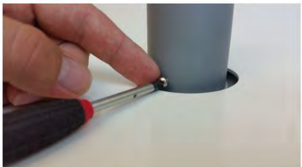
Figure 2-10 During field installation, secure the PM inlet using the retaining screws and plug in the heater
