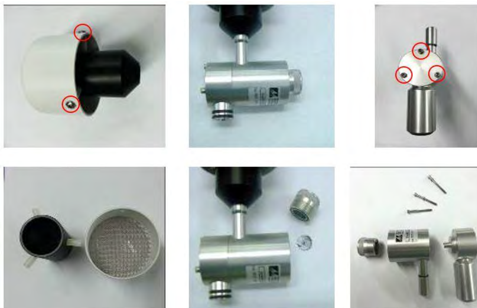
Figure 4-22 The TSP head and cyclone can be disassembled for cleaning
