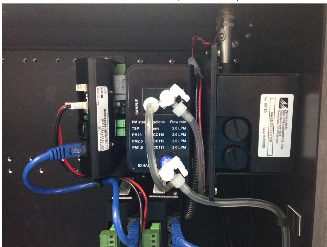
Figure 1-10 The Particle Monitor uses three modules: a) the optical engine on the far right, b) the pump module in the middle, c) the I/O module on the left
