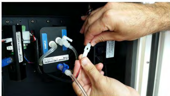
Figure 2-10 During field installation, secure the PM inlet using the retaining screws and plug in the heater
