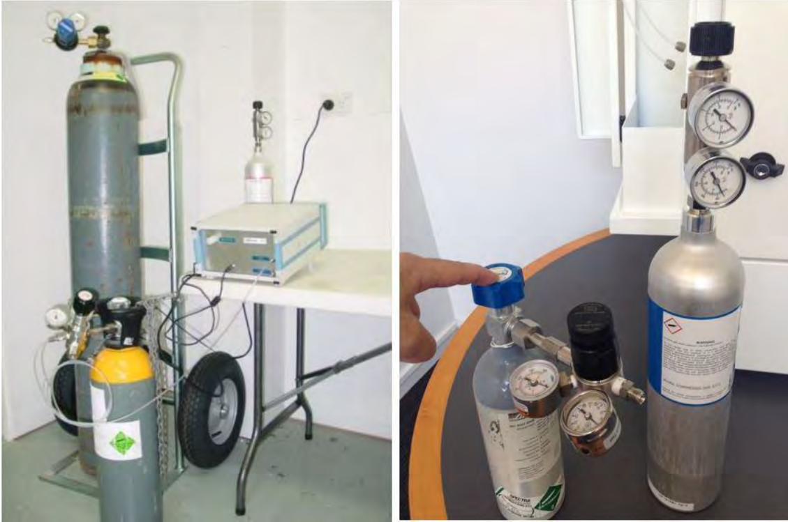
Figure 5-1 The left side image shows a large and medium laboratory gas cylinder. Both can be used with the AirCal 1000 or AirCal 8000. On the right hand side are small size cylinders from Linde and Calgaz. These are more convenient and easy to transport.
