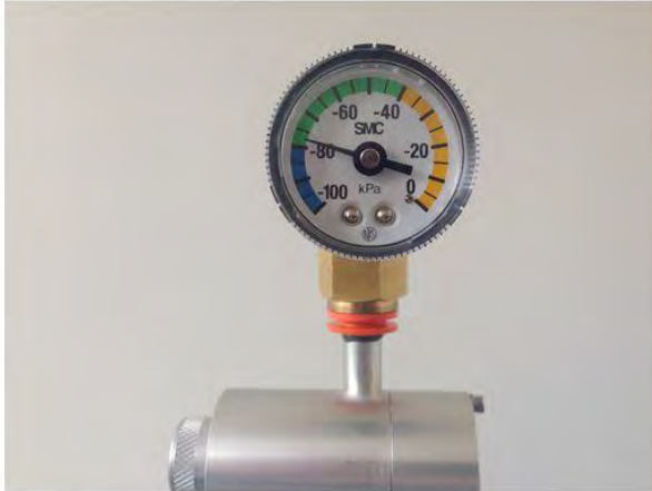
Place gauge on inlet above cyclone
