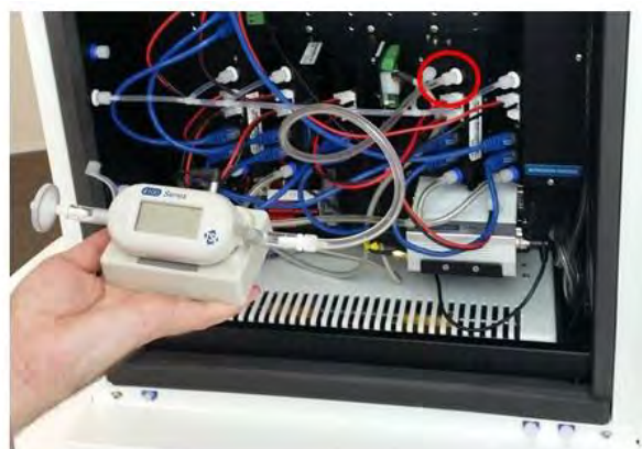
Figure 4-6 To measure the individual module flow rates, disconnect the gas inlet and attach the module inlet to the vacuum port of the R7 flow meter.
