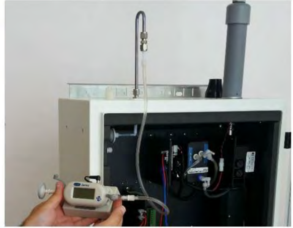
Figure 2-11 Connect inlet to AQM 65 and measure the flow rate to determine if connection is secure
