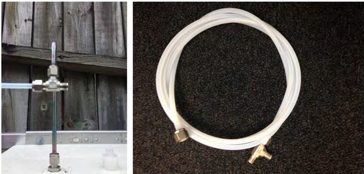
Figure 5-6 The AQM CALKIT connects the output of the AirCal 1000 to the input of the AQM 65 via a tee.
