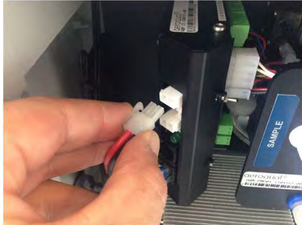
Remove power cable from electronics module
