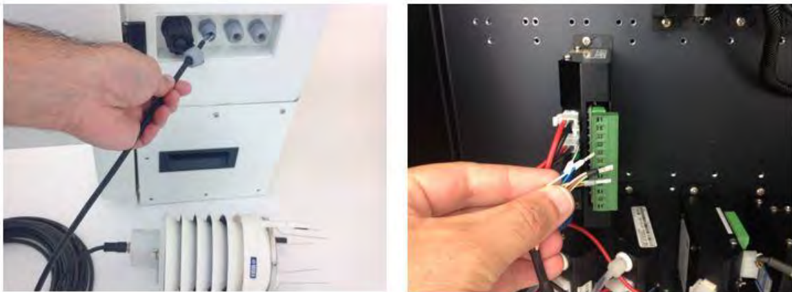
Figure 2-12 To connect third party sensors such as weather sensors, feed the cable through the gland and wire to the green plug.
