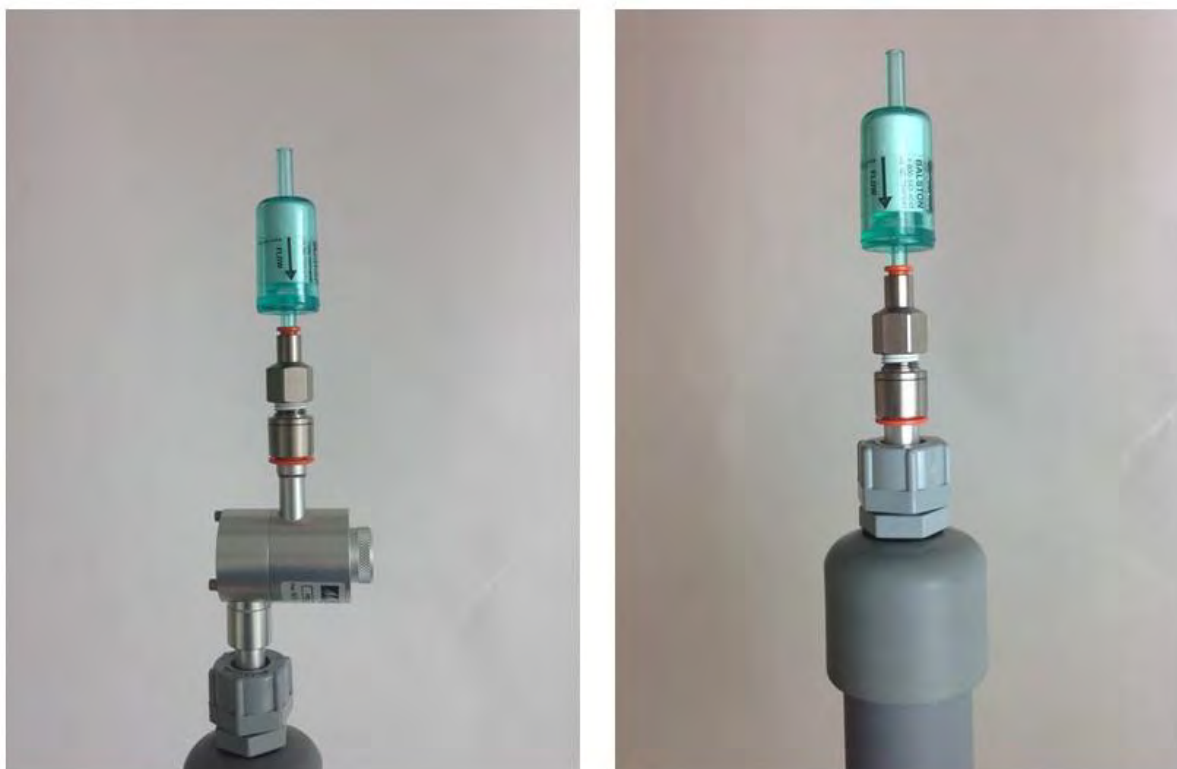
Figure 4-17 The zero filter is fitted above the cyclone for a Particle Monitor (left) and directly on the inlet for a Particle Profiler (right)
