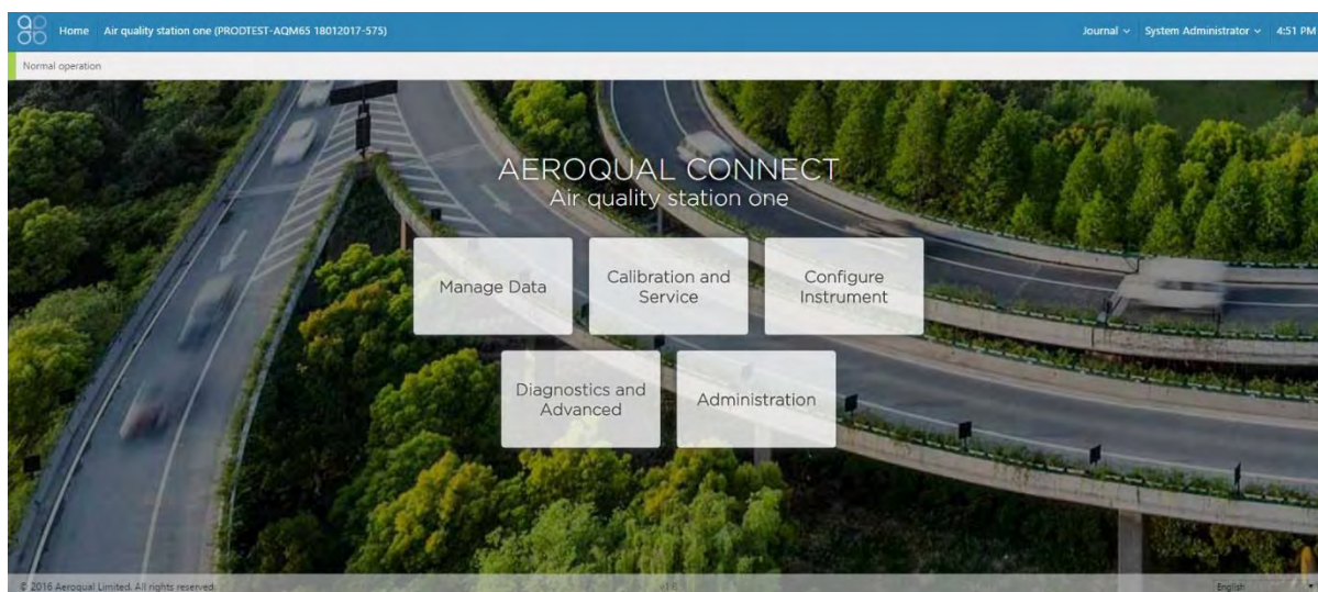
Figure 1-22 Aeroqual Connect is the operating system for the AQM 65. Aeroqual Connect is accessed using a web browser.
