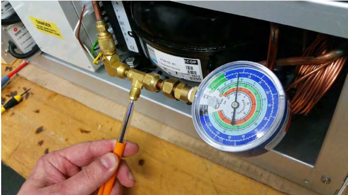
Figure 4-40 Gently release pressure from the gas line by pressing the release valve on the gauge
