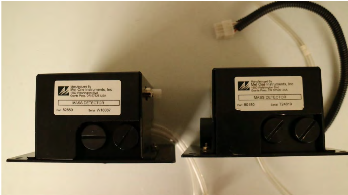
Figure 1-13 Left: 82850 optical module, Right 80180 optical module, the size and form factor are identical
