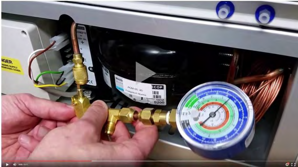
Figure 4-32 The pressure gauge provided by Aeroqual for refilling the compressor with gas
