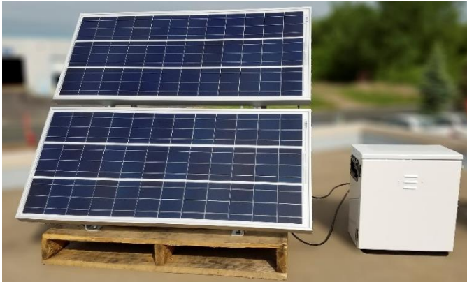
Figure 26: Solar Cell Power System
