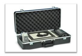
Each TE-5028A is individually calibrated on a primary standard positive displacement device (Rootsmeter) which is directly traceable to NIST.
