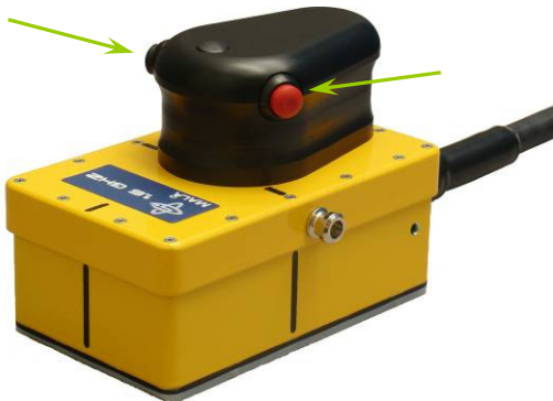
Figure 12.5 1.6 GHz antenna with the right (black) and left (red) hand buttons visible.
