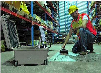
Figure 3.1 Examples of 3D/Grid Project measurements with a grid-mat.
