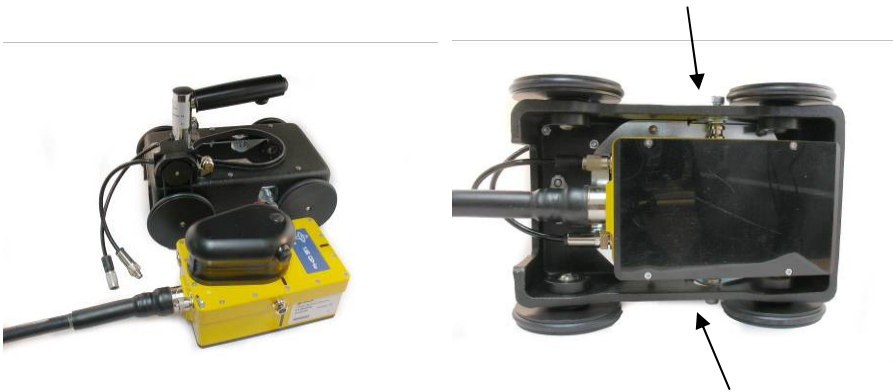
Figure 12.3 Mounting the HF antenna in the HF cart. The antenna is attached to the cart on two sides, see the arrows.
