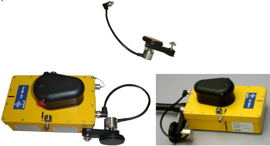
Figure 12.4 The single wheel encoder (top) and attached to a HF antenna (below) in two different directions.
