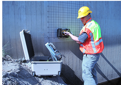
Figure 3.1 Examples of 3D/Grid Project measurements with a grid-mat.
