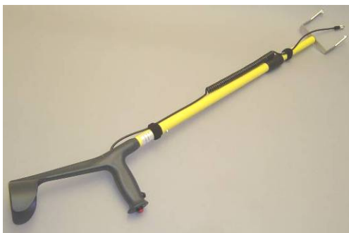
Figure 12.6 Extension pole. On the handgrip the two buttons are seen, the one on the top (red) starts a new profile.
