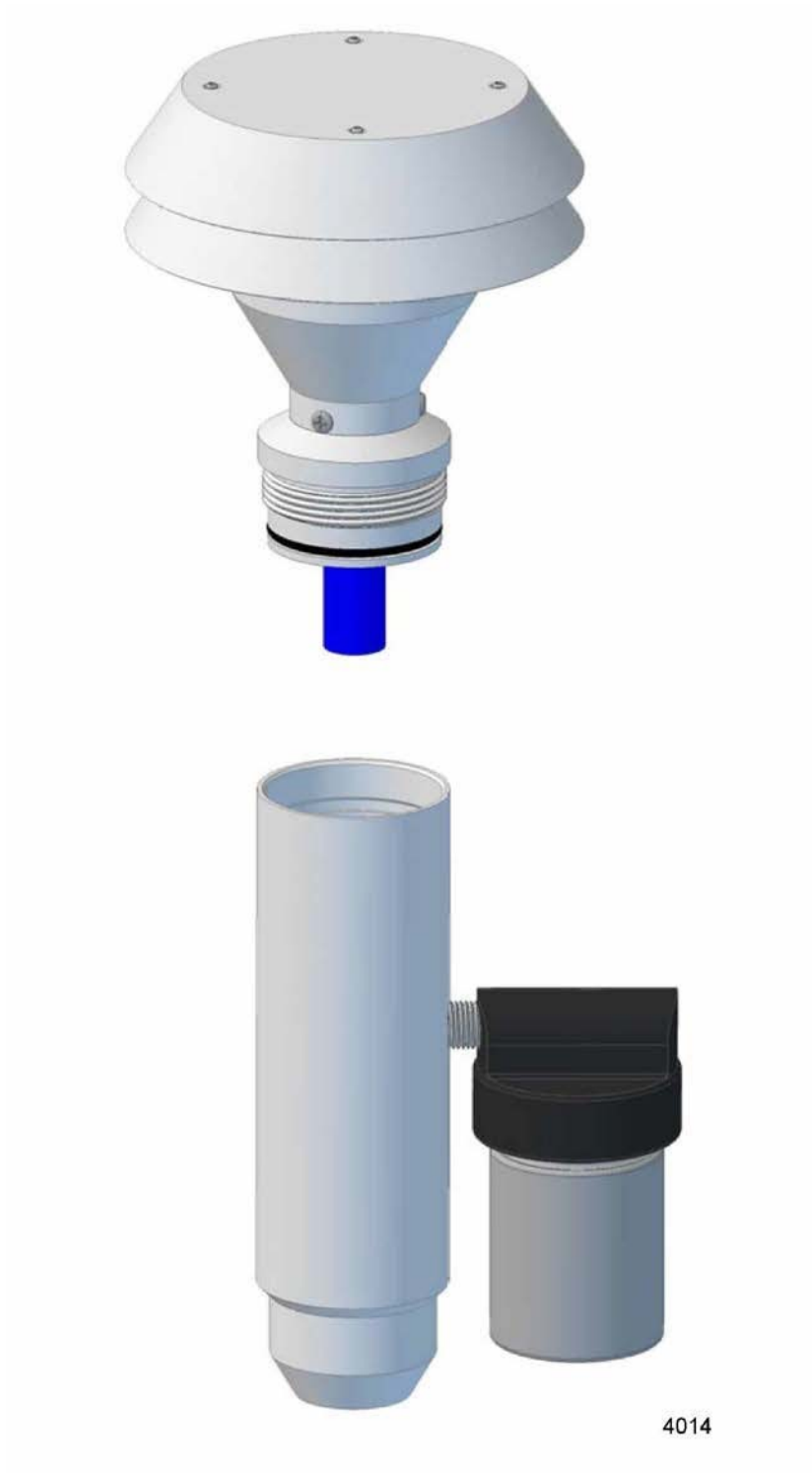
Figure 10: Initial Disassembly of Inlet
