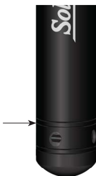
Figure 8-6 Logger Measurement Line
