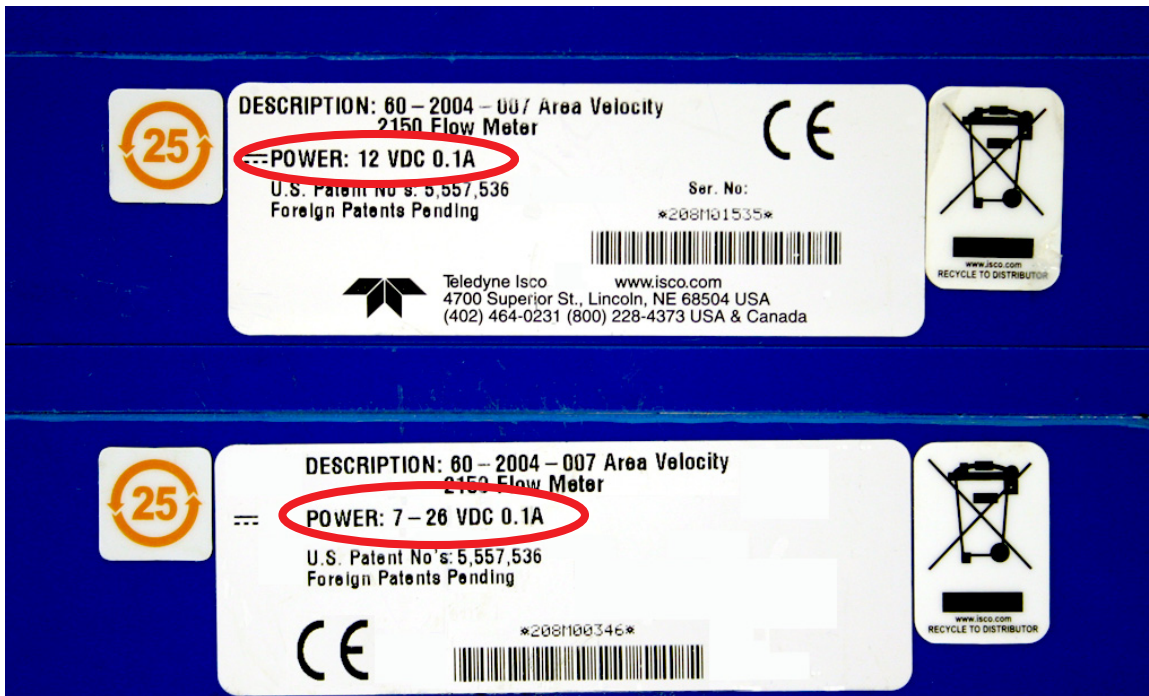
Figure 2-1 Identifying the 2150 voltage specification
