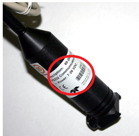
Figure 2-2 Identifying the voltage specification on the DB9 cable
