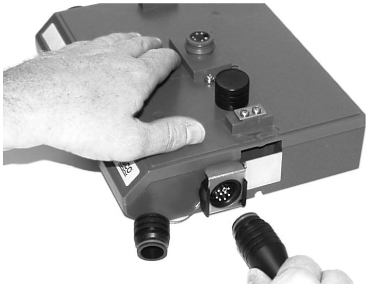
Figure 1-10 Flow Module - preparing the sensor connectors
