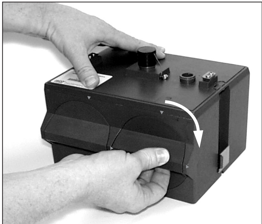
Figure 1-15 Battery Module - closing the door
