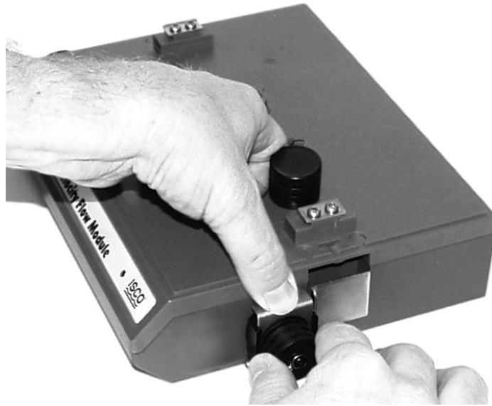
Figure 1-10 Flow Module - preparing the sensor connectors
