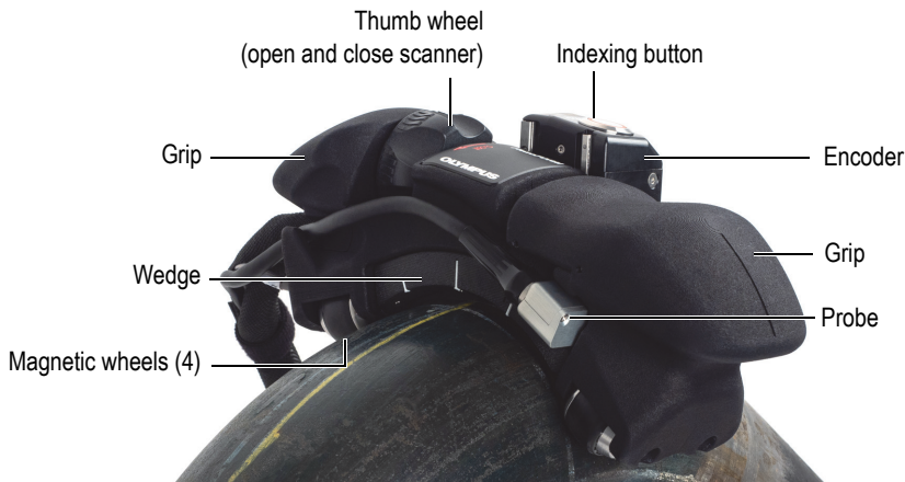
Figure 1-2 Scanner components
