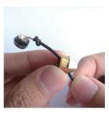
For distinguish L/R, put the masking tape on L side. (L: Green, R: Red)
