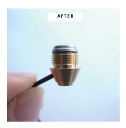
Pull the cable gently, and draw in the driver unit inside the rear body.
