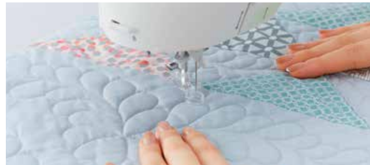
Transparent quilt presser foot makes the needle visible.
