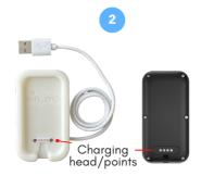
Place device in the charger (ensure the charging points on MMPSM and base match up, you will feel a magnetic pull). Charge for 2 - 3 hours
