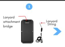
Thread lanyard string through the lanyard attachment bridge on the MMPSM, then thread the top end of lanyard through and pull tight
