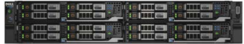
4 FM120x4 sleds in an FX2 enclosure with 2.5" drives
