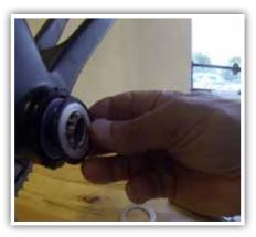
Make sure outer dust seal is in place before installing left crank arm.
