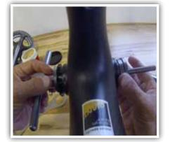
4. Use PRESS-1 or PRESS-4 with one 2437 bearing drift (drive side) and one BB86-OB-24 drift (non-drive side) to press cup into frame. Fully tighten until cup is flush with the frame.
