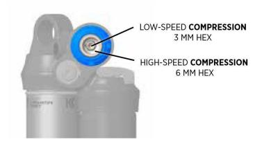
\*High-speed Compression (HSC) adjustment is useful to control shock performance during bigger hits, landings, and squareedged bumps. Turning the 6mm Hex clockwise (in) adds High-speed compression damping (firmer), turning the 6mm Hex counter-clockwise (out) reduces High-speed compression damping (softer).
