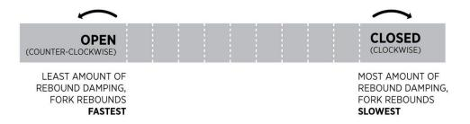
Adjust rebound until when tested, the fork returns quickly but does not top out.
