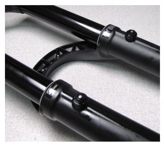
The Air Release Button at the rear of each fork leg allows the rider to equilize the air pressure between the inside of the fork lower leg and the atmosphere. This can be especially helpful at higher altitudes where the internal/external pressure differential can be its greatest.
