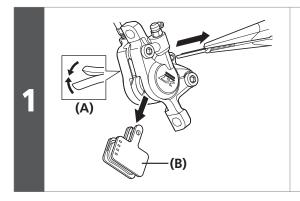
Remove the wheel from the frame, and remove the brake pads as shown in the illustration.
