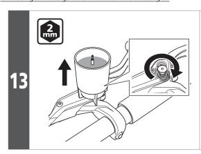
Remove the oil funnel while it is still plugged with the oil stopper and then tighten the bleed screw while letting oil flow out to make sure no air bubbles remain inside the reservoir tank.
