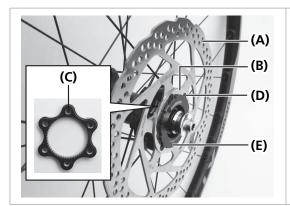
This product is an adapter used for installing 6 bolt type disc brake rotors to center lock system hubs/ wheels.
