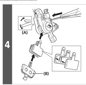
Install the new brake pads, and then install the pad spacers (red).
