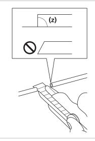
Use a utility knife or other cutting tool to cut the brake hose.
