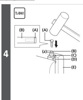
Use a tapered tool to smooth out the inside of the cut end of the brake hose, and mount the connector insert.
