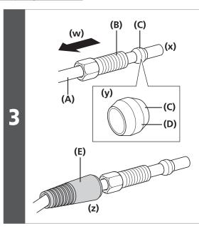
Pass the brake hose through the connecting bolt and olive.
