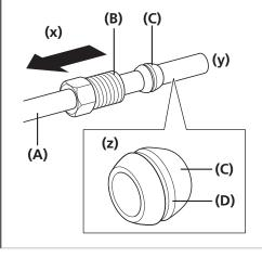
Pass the brake hose through the connecting bolt and olive.
