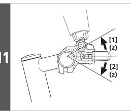
Set the lever unit to the horizontal position as shown in the illustration and tilt it 30 degrees in direction [1]; then carry out step 10 to check that there is no air remaining.
