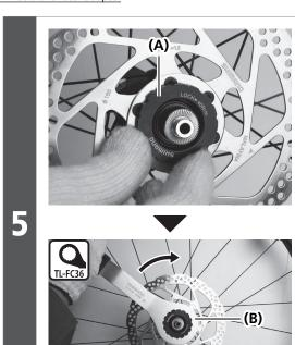
Tighten the disc brake rotor fixing lock ring.
