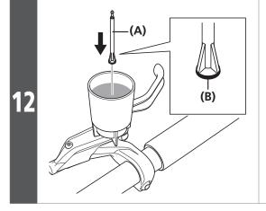
Plug the oil funnel with the oil stopper so that the O-ring mounted side is facing downward.
