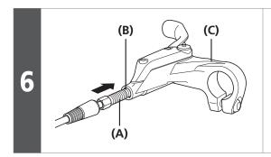
Attach the brake hose to the brake lever as shown in the illustration.
