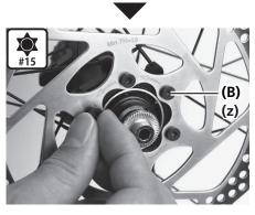
Wear gloves and turn the disc brake rotor clockwise with some force.
