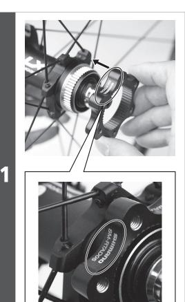
Place the disc brake rotor adapter on to the hub.
