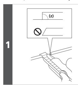
Use a utility knife or other cutting tool to cut the brake hose.
