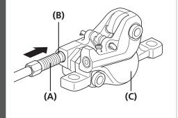
Attach the brake hose to the brake calipers as shown in the illustration.
