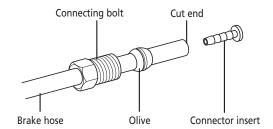
• Cut the brake hose so that the cut end is perpendicular to the length of the hose. If the brake hose is cut at an angle, fluid leaks may result.
