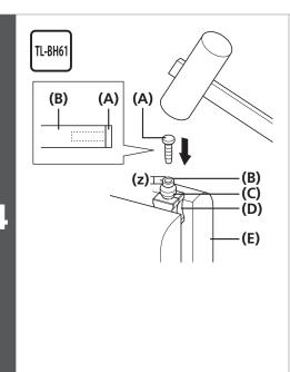
Use a tapered tool to smooth out the inside of the cut end of the brake hose, and mount the connector insert.
