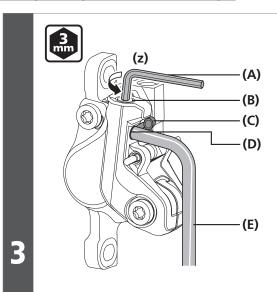
Remove the bleed nipple cap of the caliper, fill the syringe with oil, and connect the tube to the bleed nipple.
