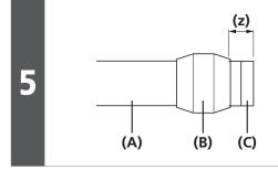
After checking that the olive is positioned as shown in the illustration, apply premium grease to the threads of the connecting bolt.
