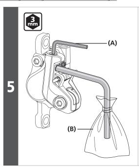
Secure the tube and bag with rubber bands, set a 3 mm hexagon wrench as shown in the illustration, and connect the tube to the bleed nipple.
