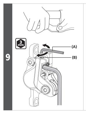
With the brake lever depressed, open and close the bleed screw in rapid succession (for approximately 0.5 seconds each time) to release any air bubbles which may be in the brake calipers.
