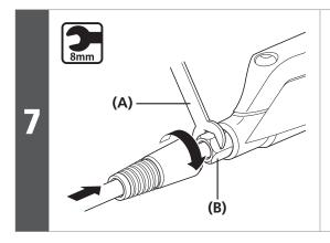
While pushing the brake hose, tighten the connecting bolt.
