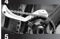
Install the crankset and chain. Close the upper guide and reinstall the upper guide bolt. Tighten the upper guide bolt to 1.2-1.3 Nm. The backplate features laser etching to assist in the vertical positioning of the guide. There should be roughly 3mm of space between the chain and the ceiling of the upper guide.
