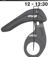
Adjust the guide so that the upper guide bolt is located between 12:00 and 12:30 relative to the center of the BB. Once there, tighten the ISCG screws to 8-9 Nm or BB cup (for BB-mount guides) to its recommended torque.
