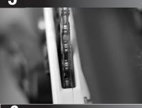
Check that the alignment of the guide is correct. The chain should be centered in the upper guide in the middle range of the cassette. There should be little or no contact between the chain and upper guide while in the smallest or largest cogs of the cassette. Refine this spacing using the included ISCG spacers or 1mm BB spacer (for BB-mount guides) if necessary.\*
