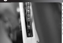
Check that the alignment of the guide is correct. The chain should be centered in the upper guide in the middle range of the cassette. There should be little or no contact between the chain and upper guide while in the smallest or largest cogs of the cassette. Refine this spacing using the included ISCG spacers or 1mm BB spacer (for BB-mount guides) if necessary.\*
