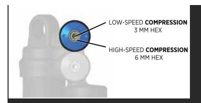
\*High-speed Compression (HSC) adjustment is useful to control shock performance during bigger hits, landings, and squareedged bumps. Turning the 6mm Hex clockwise (in) adds High-speed compression damping (firmer), turning the 6mm Hex counter-clockwise (out) reduces High-speed compression damping (softer).
