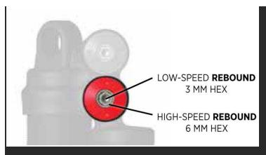
\*High-speed Rebound (HSR) adjustment is useful to allow the shock to recover from bigger hits and square-edged bumps quickly enough to absorb consecutive hits. Turning the 6mm Hex clockwise (out) speeds up High-speed rebound.
