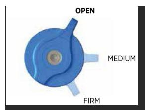
\*OPEN Mode Adjust: Open mode adjust is useful to control fork performance under rider weight shifts, G-outs, and slow inputs. OPEN mode adjust provides 22 additional fine tuning adjustments for the OPEN mode. Setting 22 will have a more plush feel and setting 1 will have a firmer feel.
