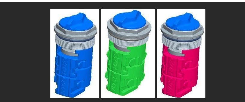
Some 32mm FLOAT forks come with a factory installed hollow volume spacer pictured below. Standard blue 32mm volume spacers can be added to the hollow volume spacer to further reduce air volume if desired.
