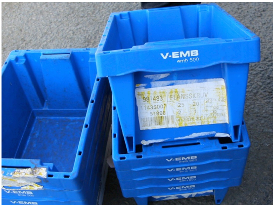
Figure 6.4. Plastic box with label difficult to remove.
