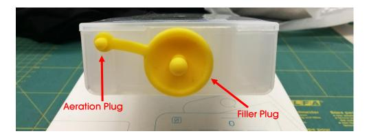
In order to allow the air to escape and the ink to 'calm down', hold the cartridge upright after filling (aeration plug still removed!) and shake it gently about 10 times. Leave the cartridge upright for about 5 minutes.
