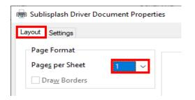
In the "Layout" tab you can specify how many pages of the PDF should be printed on **ONE** sheet. The standard value is "1".
