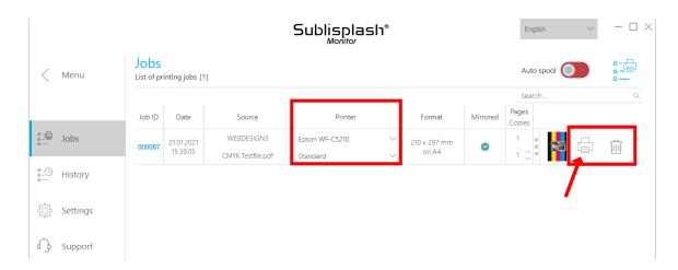
In the "**Printer**" section, you can now change the printer and/or the print profile. You can delete the print job by clicking on the "**Trash**" icon.
