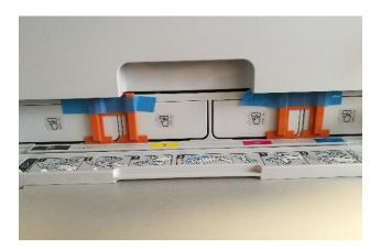
The next step is to fill the empty cartridges supplied. When filling the cartridges, it is essential to fill the **correct** ink colour in the **corresponding** colour tank! The empty cartridges are marked with a sticker indicating the colour to be used. The colour abbreviations are as follows:
