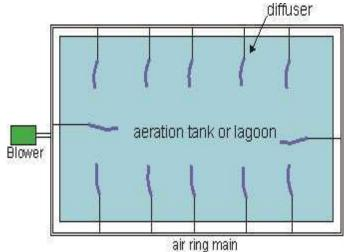
When air is compressed it gets hot, for every 0.1 bar, the air temperature will increase by 10°C. The maximum upper temperature for plastic pipe is 90°C. If the temperature is likely to exceed 80°C then metal pipe is recommended.
