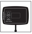
**STEP 5: TEST** Connect the male end of the light string into the female end of the Solar Panel cord. On the back side of the solar panel, turn the switch to "ON" Then, test the bulbs by covering the solar panel with a dark towel (to activate the sensor). Check each bulb to see that itis lit up. If not, adjust tension on bulb, or try another bulb.
