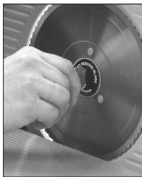
Figure 7. Turn the screw clockwise for blade removal.
