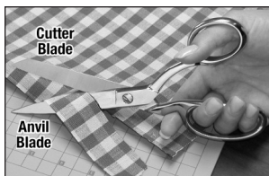
Figure 2. Typical position of the Cutter Blade and Anvil Blade on right-handed scissors.
