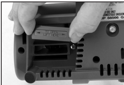
Figure 15. Removing cover under base to clean out metal dust (see Normal Maintenance section).
