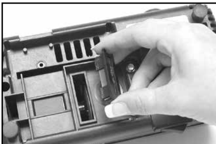
Figure 14. Removing cover under base to clean out metal dust (see Normal Maintenance section).
