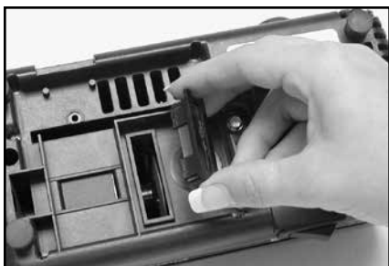
Figure 11. Removing cover under base to clean out metal dust.
