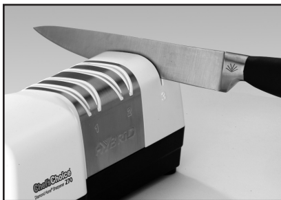
Figure 6. Knife in Stage 3. Use back and forth sharpening strokes with light downward pressure. See text.
